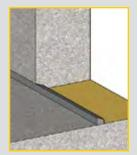
Krystol technology delivered through a slurry treatment and external waterstop that ensures permanent waterproofing protection.
