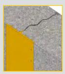
Kryton's Crack Inducing Waterstop creates a controlled crack, then introduces Krystol technology through an externally placed waterstop that ensures permanent waterproofing protection.
