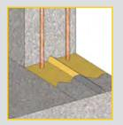
Krystol technology delivered through an internally placed, triangle shaped, waterstop and a slurry treatment that ensures permanent waterproofing protection.
